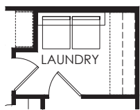
Dual Washer/ Dryers
